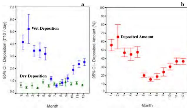
Figure 2: Month-to-month variability at 95% confidence interval of averaged dry and wet deposition patterns (in tonnes per day) and (b) deposited amount (in %) resulted from the Severonickel continuous emissions.
