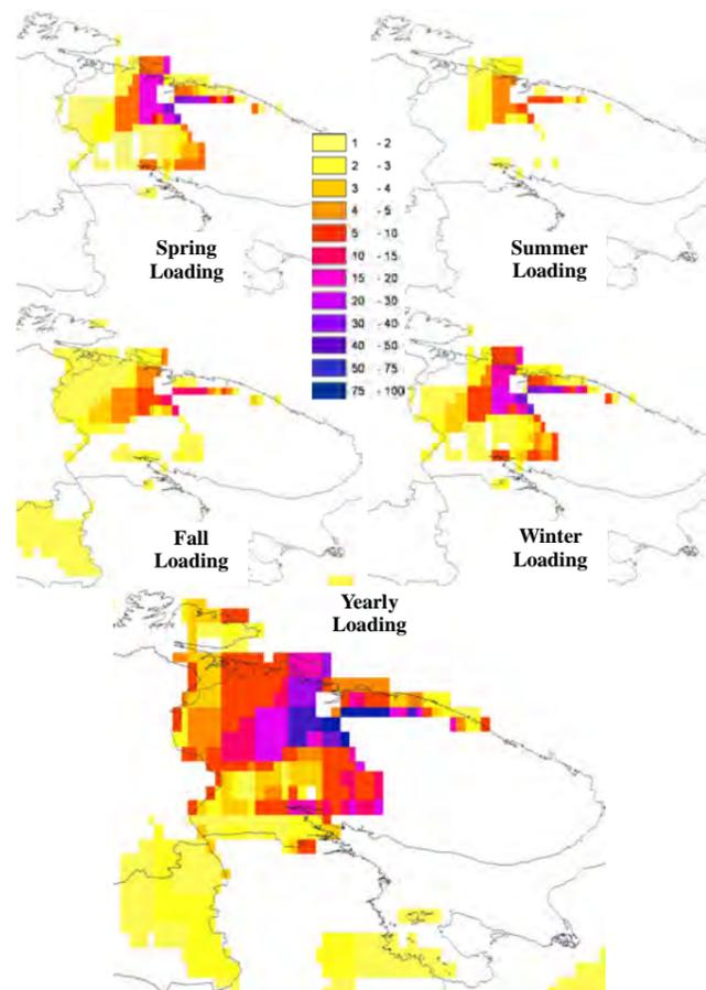
Figure 4: Seasonal variability of individual loadings for population (in kg/person) from deposited sulfates resulted from the Severonickel smelters continuous emissions (mild scenario).
