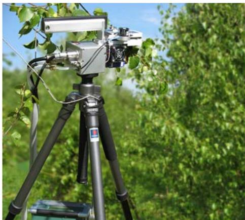
Fig. 2. The LI-6400XT Portable Photosynthesis System at a forest experimental plot
